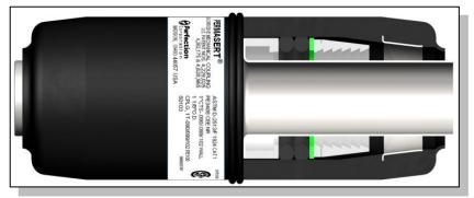
diameter of the tubing, again, compressing the tubing wall to the oring creating a gas seal.
