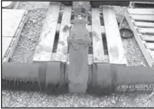
Figure 21 Ductile Iron Gate Valve with PE Ends
