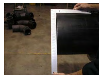
Figure IV-b - Measuring allowable gap with Carpenter's Square
