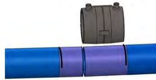
Step 1 - Measure and scrape one end for the full length of the coupling, measure and scrape the other end for 1/2 the coupling length. Remark stab depths after scraping if necessary.
