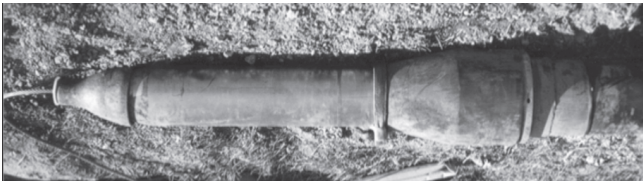
Figure 2 The Bursting Head of the Pneumatic System
