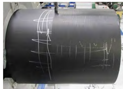
Figure V-d – Inadequate Removal of Witness Marks
