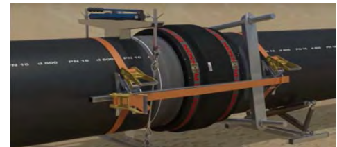
Figure III-d - Mechanical Pulling Tool
